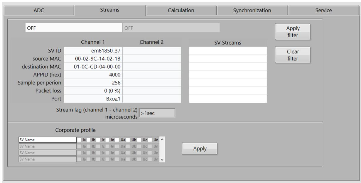
When external streams are present at the EXT input of the EM61850, the names of the streams will be automatically displayed in the list **SV Streams**.
