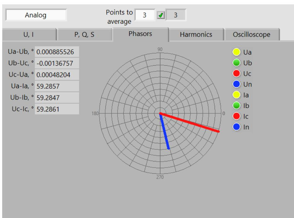
The tab “**Phasors**” displays numeric values of phase shifts among signals in the channels. The vector diagram shows phasors (angles with respect to PPS).
