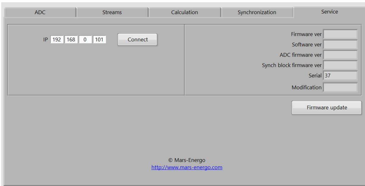
Click “**Connect**” to activate the program on the instrument with the specified **IP** address.
