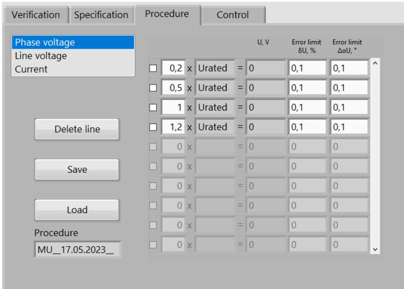
The tab is optional, and its fields can remain empty. However, with these fields the user can specify a verification procedure as a set of test points, save it to a file with the “**Save**” button and then activate it at any time with the “**Load**” button, if necessary. Then, if specified, these test points are displayed in the Verification tab as pop-up tips for signals to be applied to the tested device.
