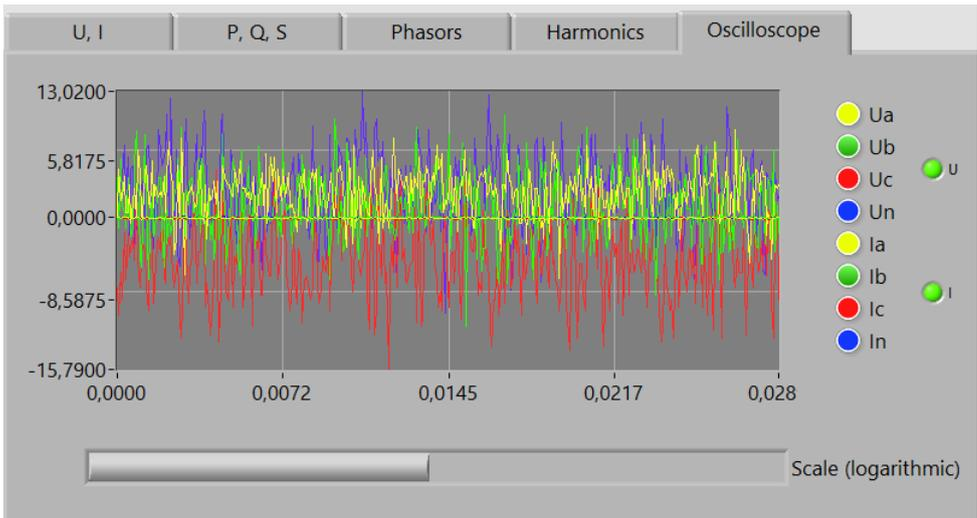
In the **Oscilloscope** mode, the waveforms on the selected channels (based on the measurements over the latest second) are displayed. At the leftmost position of the logarithmic scaling slider the amplitudes within 0 to 0.001 s are plotted. By moving the slider to the rightmost position you can view the complete 1-second curves.
