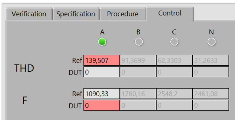
The Control menu is used to keep watch on signal quality by monitoring such parameters as total harmonic distortion (THD) and the difference in frequencies of the tested and reference merging units (F). The parameters are highlighted, if their values fall outside the permissible range. Verification is useless and cannot be performed if THD is more than 5% and F is more than 0.001 Hz. Please note that the quality is checked just for the channels marked in the verification tab.
