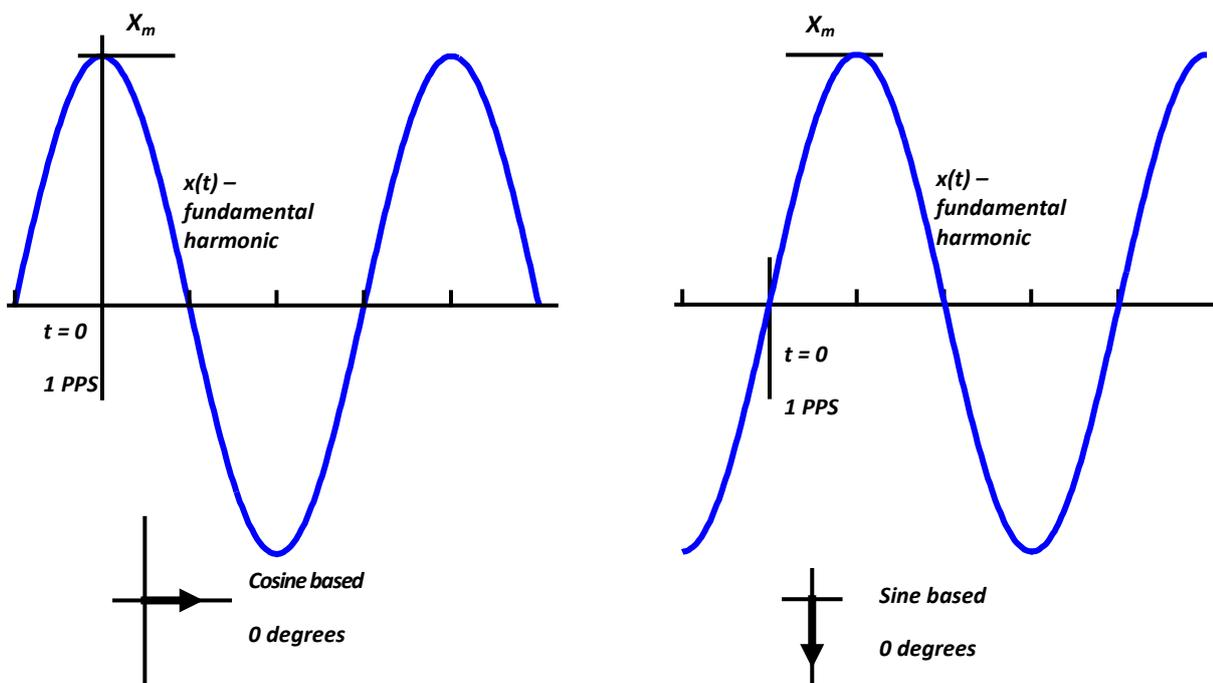
**Cosine based:** the phase offset is assumed to be zero, if a time stamp (at the moment of going from one UTC second to the next) matches the curve of the fundamental signal harmonic at its maximum
