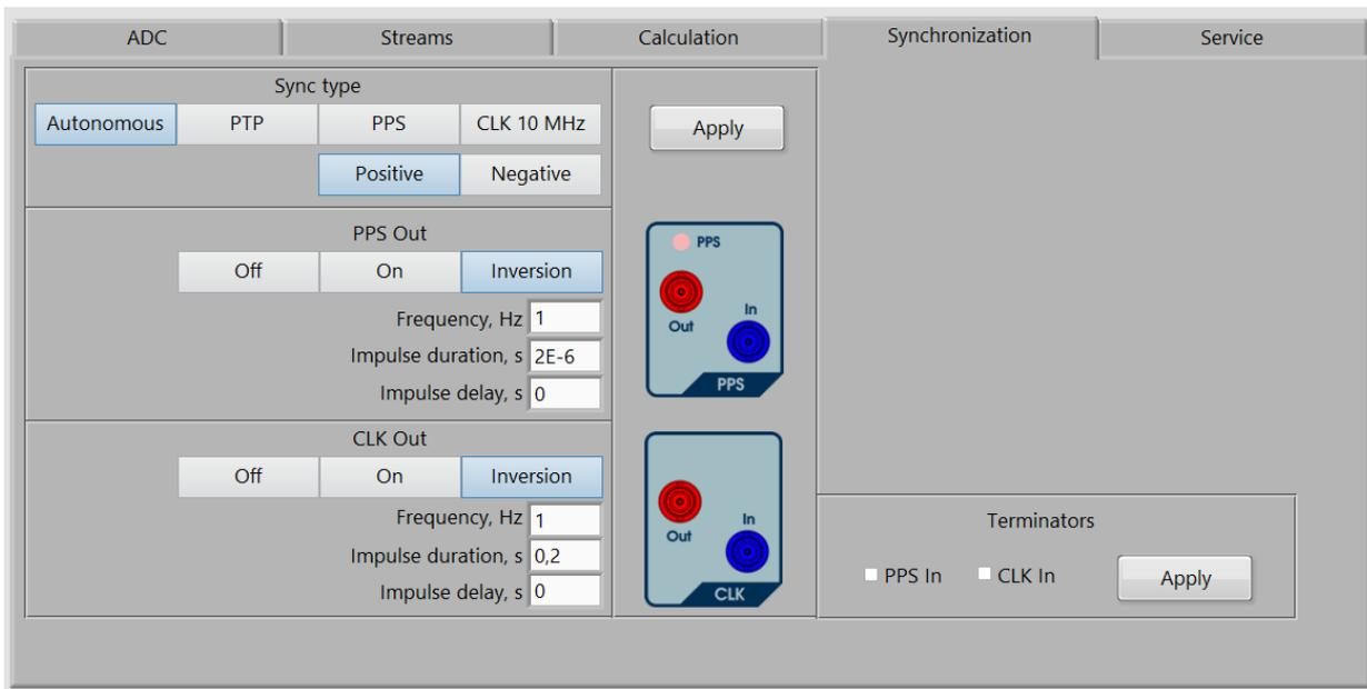
Two types of synchronization are available: internal and external.
