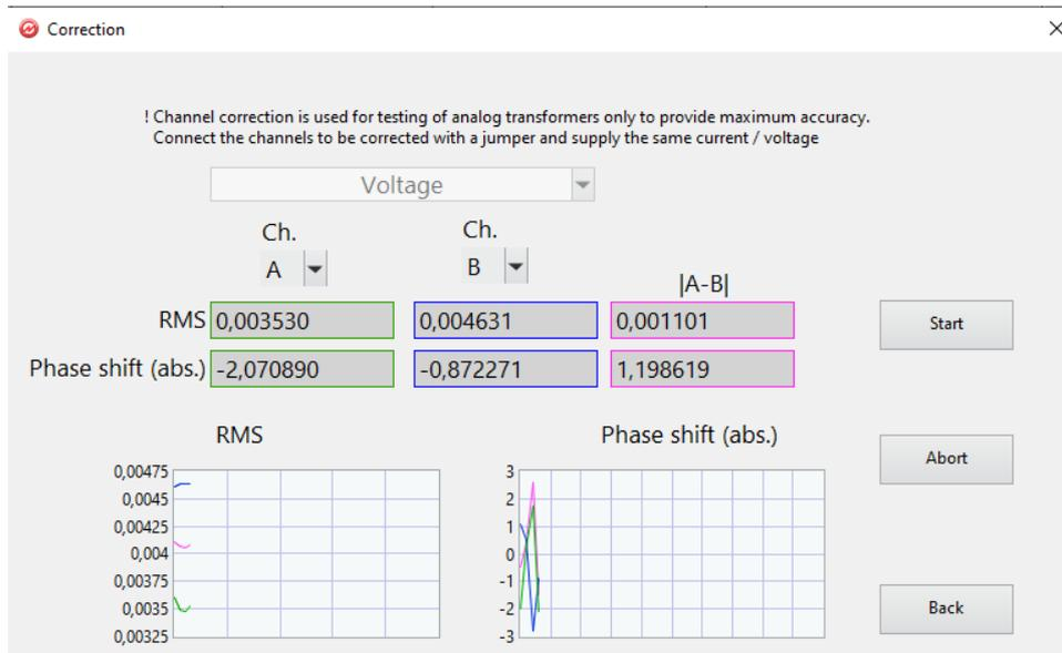
The correction of channels is only performed prior to testing of conventional current or voltage transformers. It should be performed in 30 min (or later) after applying power to the EM61850.
